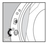
To disable this device and restore the possibility of closing the door, rotate the button anti-clockwise until the groove is vertical.
